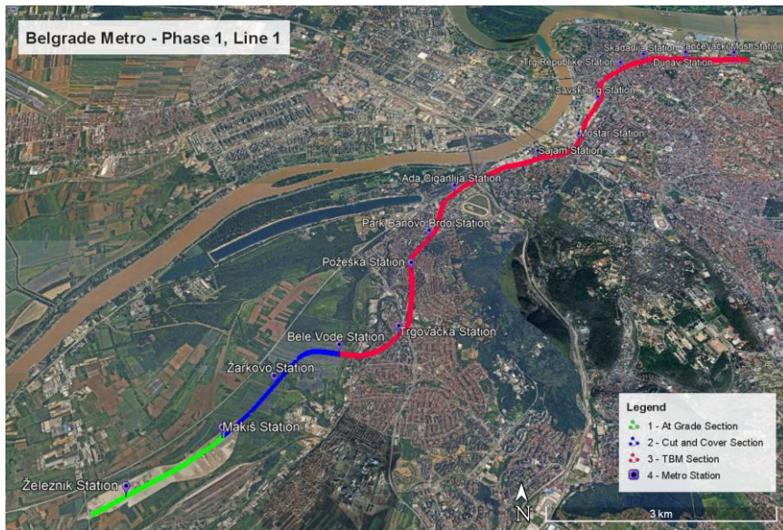
Fig. 1. Route of Phase 1, Line 1 of the Belgrade Metro, showing sections and stations.
