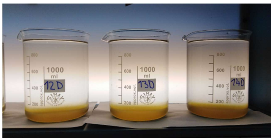
Figure 8. JAR 2 additional Samples 12D, 13D and 14D after settling.
