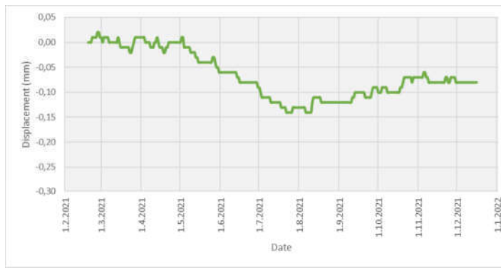
Figure 12. The diagram of crack behavior (deformer D-4V)
