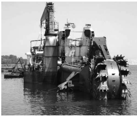
Figure 9 Dredge with buckets shown (photo documentation of Kovin mine) [12]
