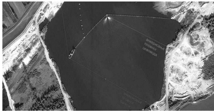
Figure 10. Anchoring of pipelines and dredgers (photo documentation of Kovin mine) [12]
