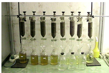
Figure 1. Laboratory experiment to study the migration ability of stable strontium (Sr) in the soil (photo by A. Lavrishchev)
