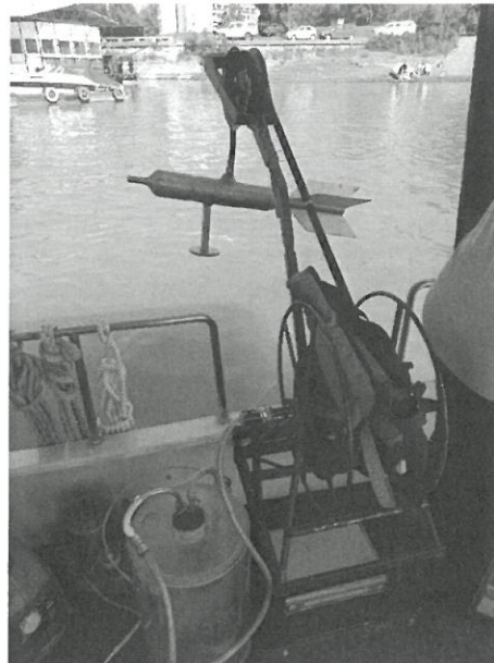
Figure 4. Devices used for suspended sediment sampling (pump sampler).
