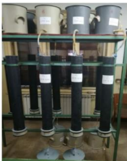
Figure 2 Apparatus for percolation leaching
