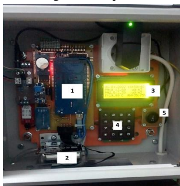
Figure 1 AMS/2022 module layout inside the housing (1. Control module, 2. PM module, 3. LCD module, 4. Keyboard, 5. ON/OFF switch)
