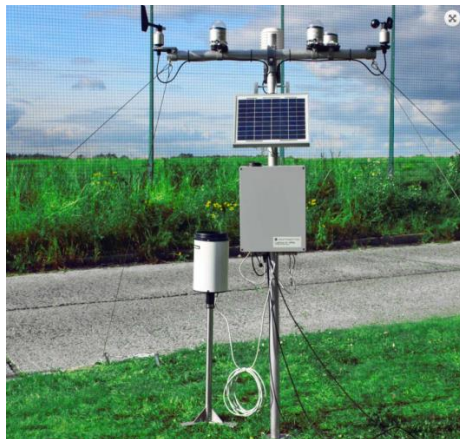
Figure 1 Automatic weather station with solar power supply produced by UIT -gmbh [3]
