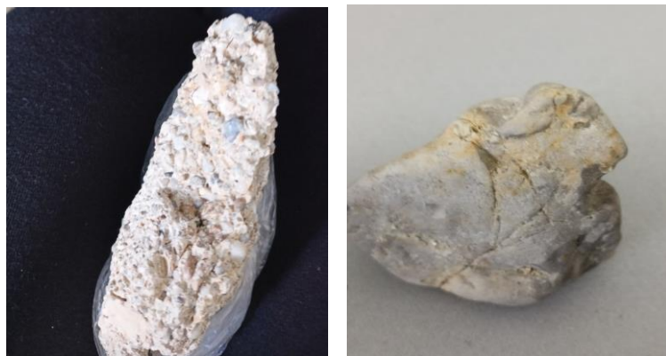
Figure 2 Fragment of pebble sandstone with calcite binder 75/125 mm (left) and sandstone clast-SiO 2 binder in pebble sandstone 32/63 mm (right)
