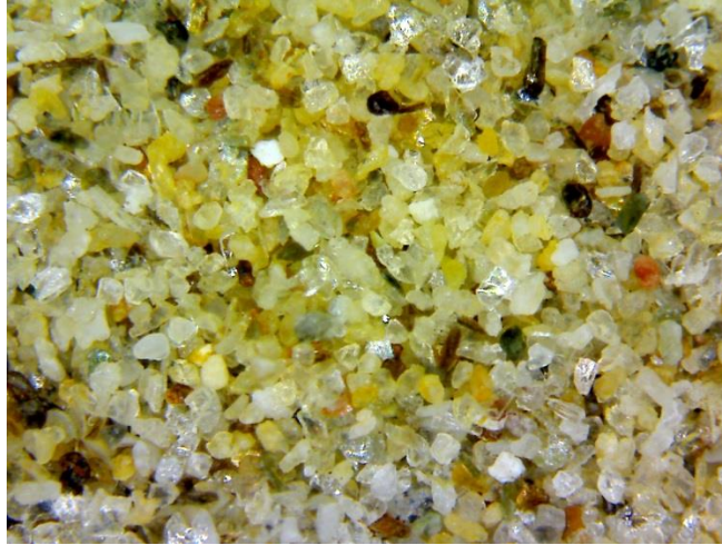
Figure 3 Microscopic appearance of fraction 0.250 / 0.125 mm, binocular magnification 40X [7]
