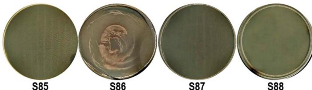
Figure 24. Screening from microbial strain resistant to  $\text{Cu}^{2+}$  100mg/L – isolates from samples collected in July 2021
