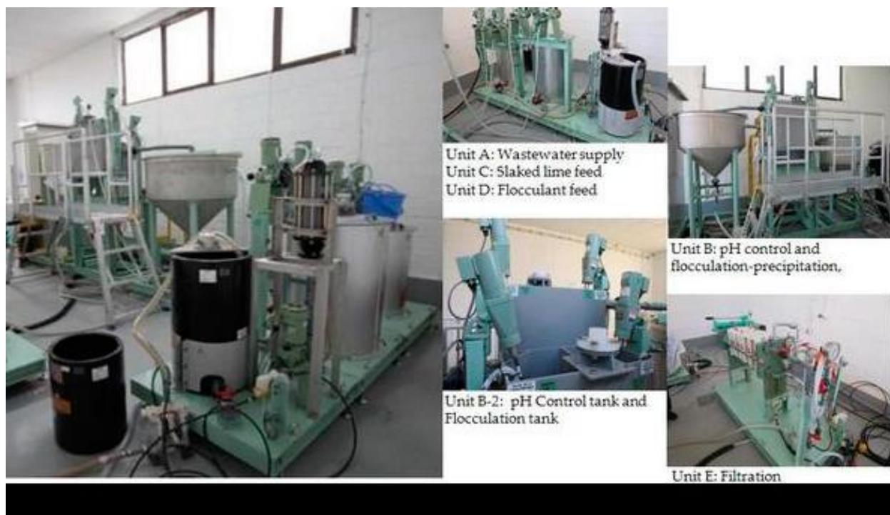
Figure 2. Semi industrial plant for two-step neutralization treatment
