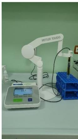
Figure 11. Mettler Toledo SevenCompact™ S220 Millivoltmeter
