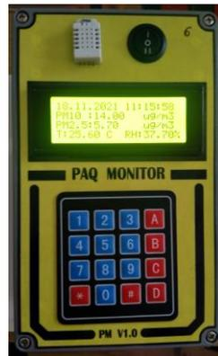
Figure 12 Using the LCD display in a portable measurement device
