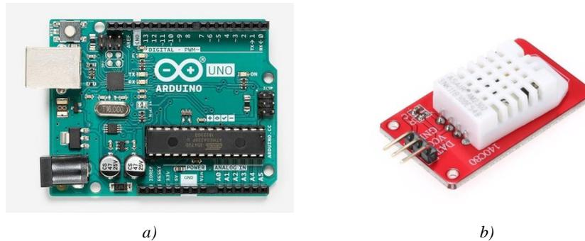
**Figure 1** a) Arduino Uno microcontroller board, and b) DHT22 sensor
