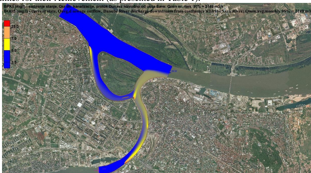
Figure 2. Wastewater discharges from BCSS (current state) into the Sava and Danube Rivers upstream from the confluence (average wastewater flow, low waters, dry period), BOD 5 [1]
