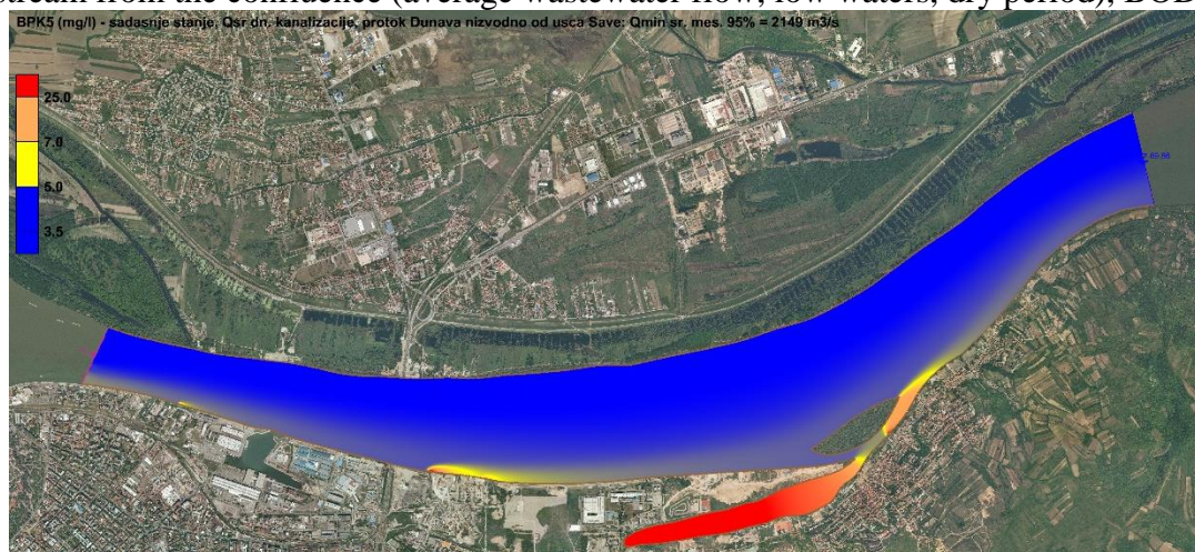
Figure 3. Wastewater discharges from BCSS (current state) into the Danube River downstream from the confluence (average wastewater flow, low waters, dry period), BOD 5
