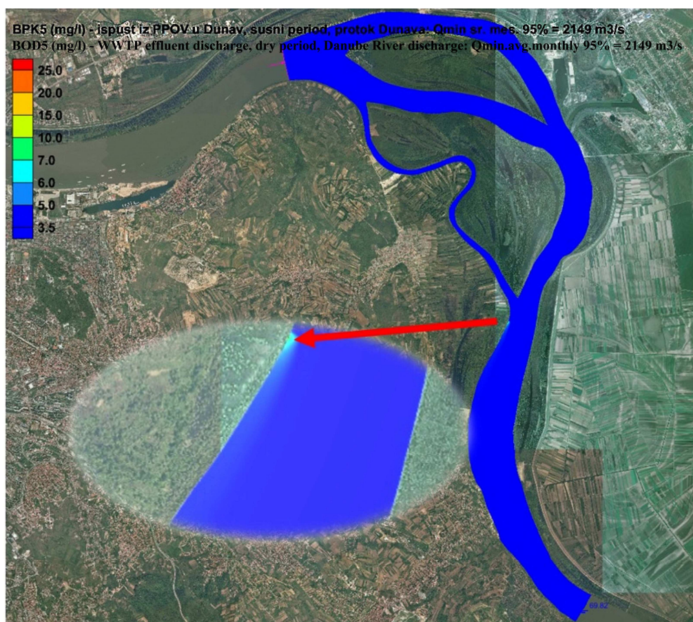
Figure 12. Effluent discharge from WWTP "Veliko Selo" into the Danube River (average effluent flow, low waters, dry period)
