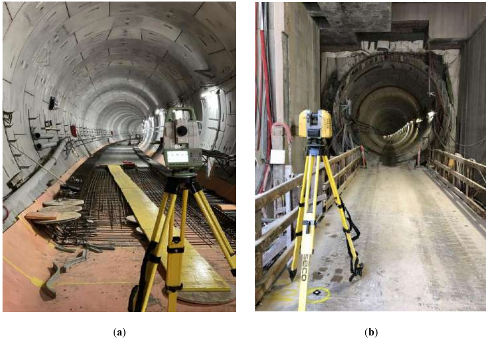
Fig. 1. Measuring technologies used in the project: (a) Leica TS16 total station for geodetic control network establishment, (b) Topcon GLS-2000 terrestrial laser scanner for detailed 3D data acquisition.
