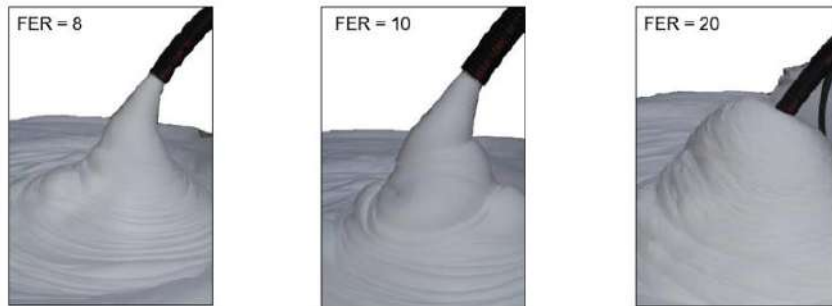
Fig. 2. Example of one foam at same Cf expanded at three different FER (Source: Sposetti, 2023).
