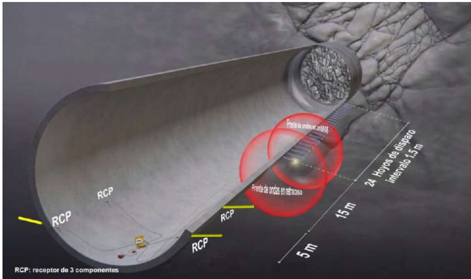
Fig. 1. Standard layout when using the TSP 303 technology consisting of an array of 24 shot points and four 3-component receivers are installed as close as possible to the tunnel face.
