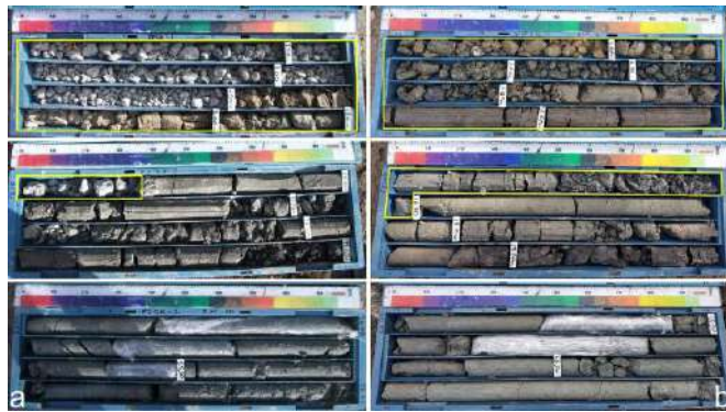
Fig. 5. Photographs of core boxes from the drillings at the T1 Tunnel Portal entrance (a: YTSK-1; b: YHSK-3 drillings, the area within the yellow lines shows the landslide material; Fugro-Sial, 2020).
