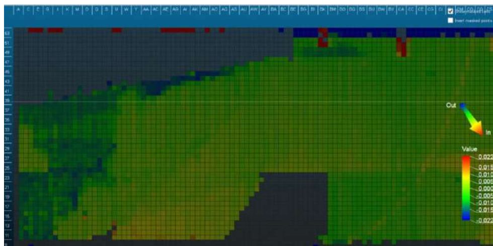
Fig. 7. Comparison of actual vs. reference geometry of atrium walls, visualized through OPSIS.
