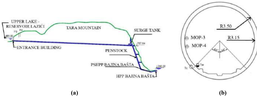
Fig. 2. (a) Longitudinal tunnel profile with a schematic view of the upper lake, pipeline, PSHPP and HPP “Bajina Bašta”, (b) Cross-section of tunnel (Radovanović et al., 2022).
