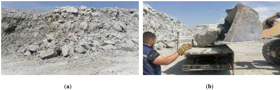
Fig. 1. (a) Position of a bench from which the rock mass block was extracted; (b) loading of the rock mass block.
