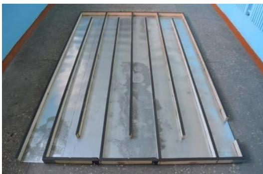
**Fig. 3.** View of the middle chamber of the combined heat exchanger
