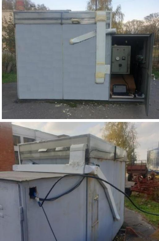
**Fig. 2.** General view of the dryer with a combined heat exchanger
