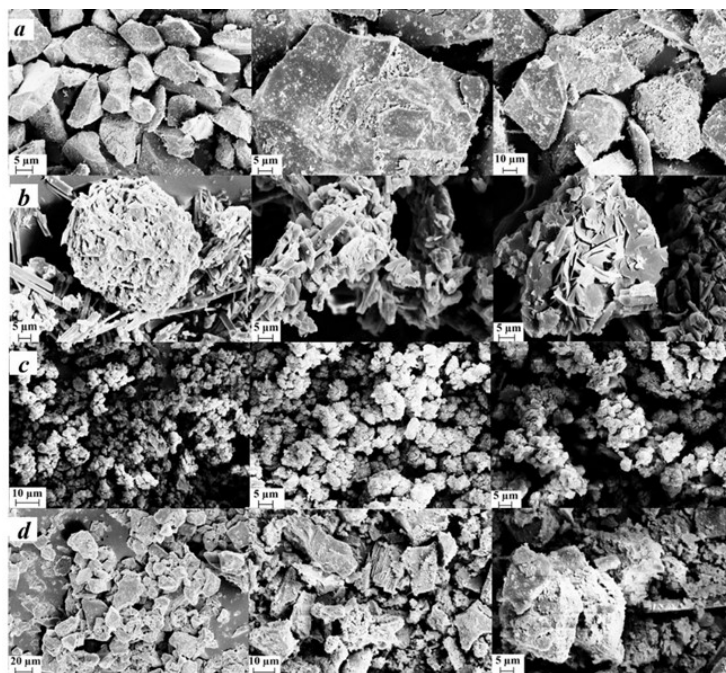
Figure 4 SEM-images of the Nud II ore particles (a), mixture of Nud II ore with ammonium sulfate (b), roasted mixture of Nud II ore and ammonium sulfate (c), residue after water leaching of the roasted mixture (d)
