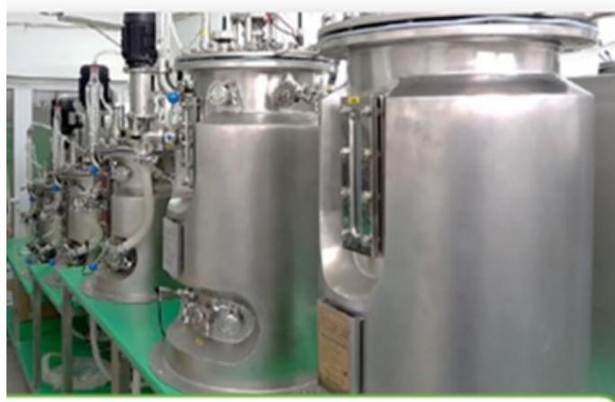
Figure 11 Integrated bioleach Pilot plant facility, capacity 20L pulp/day
