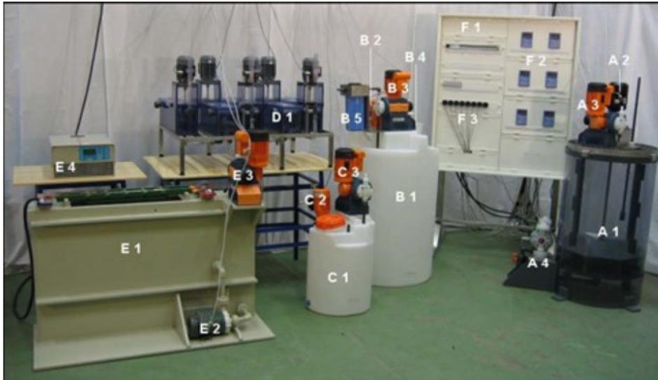
**Figure 13** Laboratory plant for leaching, solvent extraction and electrowinning
