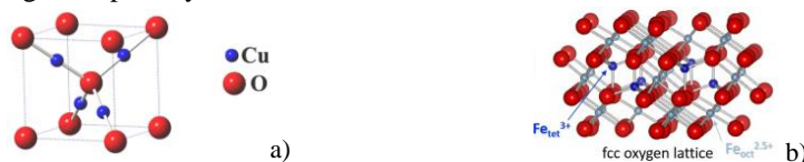
Figure 4 Unit cells and densities of: a) Cu 2 O; \rho=6.0\text{g/cm}^3 ; and b) Fe 3 O 4 –magnetite; \rho=5.17\text{g/cm}^3 [12]
