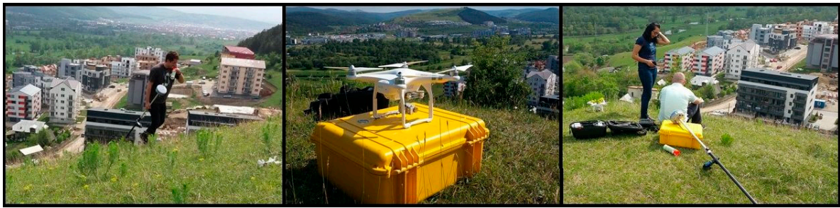
Figure 10. Ground control points (GCPs) and CPs GNSS RTK measurement and unmanned aerial vehicles (UAV) mission preparations.
