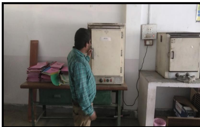
Fig. 2 Measurement of moisture content of wheat seed grain sample by oven dry method
