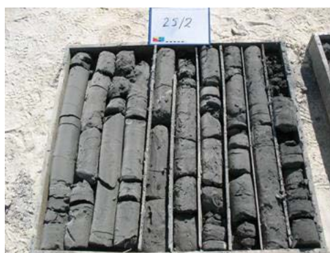
Figure 3 - Core of technogenic raw material from the old flotation tailing pit - Bor
