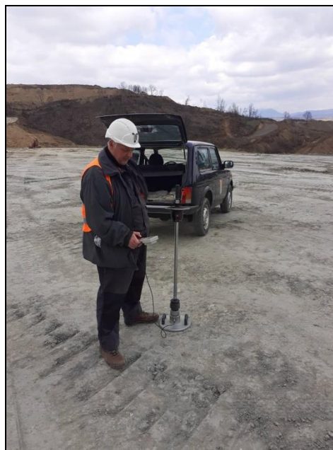
Figure 2 Performing a dynamic plate load test (light falling weight device)
