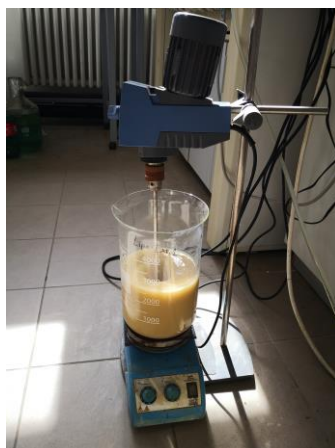
Figure 2. Experiment leaching of gold on laboratory equipment
