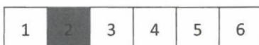
Figure 3 Schematic representation of the location from which the 2/2 ( \perp ) sample was cut from the ingot
