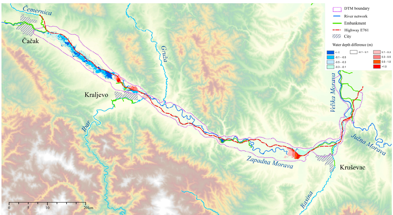
Figure 20. Difference between the levels of future and existing state of highway construction
