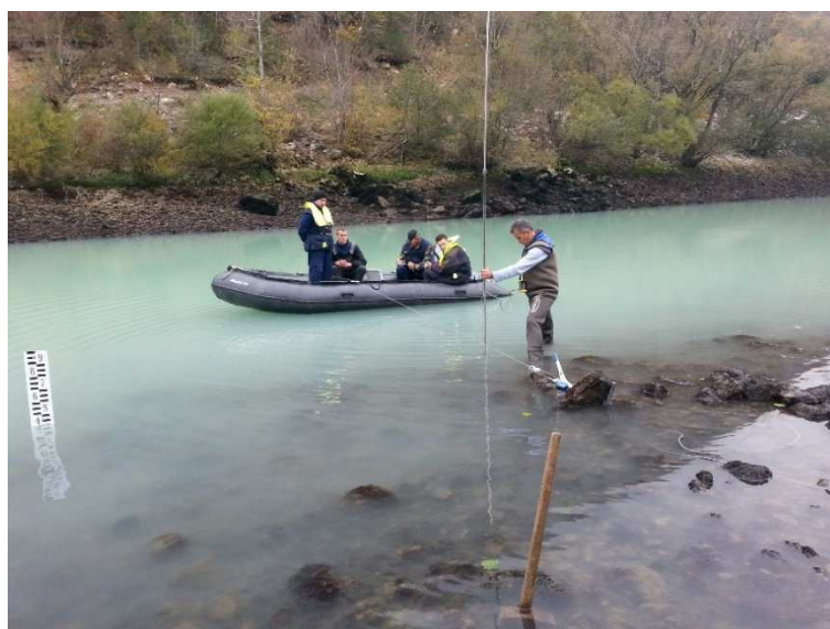
Figure 25. Hydrometric measurement of total seepage downstream of the dam
