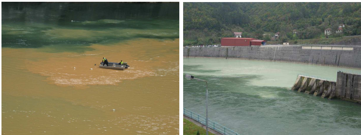
Figure 23. Visual observation of the source downstream of the dam (removal of clay and grouting mass) and sampling
