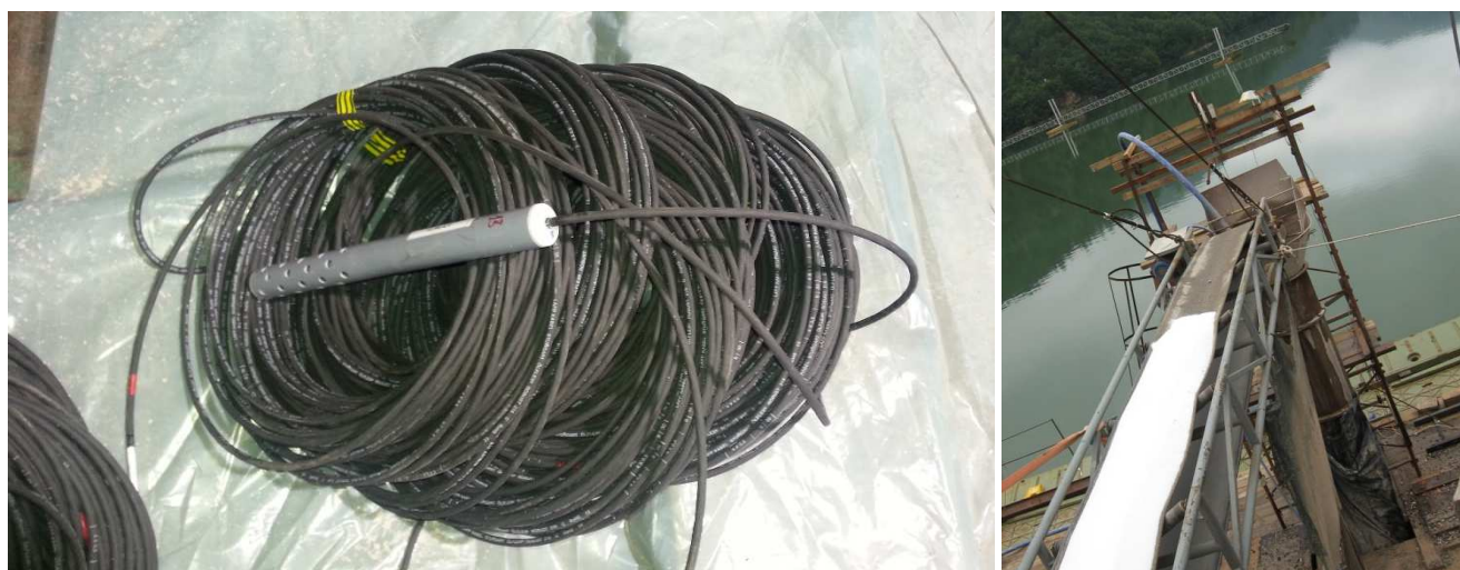
Figure 21. Electrical conductivity measuring probe, NaCl tracer test
